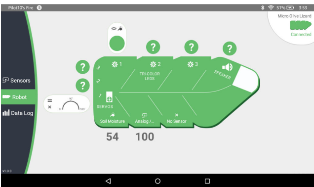
Fig. 3. Screenshot of the Flutter app as used in Pilot 3. This screen allows students to configure relationships between inputs and outputs. Clicking on one of the question marks opens a control panel (Fig. 4).
